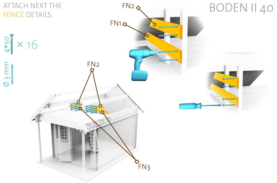
SAW THE FENCE DETAILS INTO THE RIGHT SIZE AND SHAPE, ATTACH WITH SCREWS.
