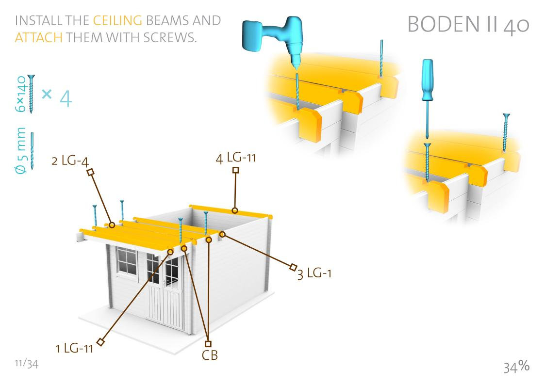
INSTALL THE BEAM AND **ATTACH** WITH SCREWS.
