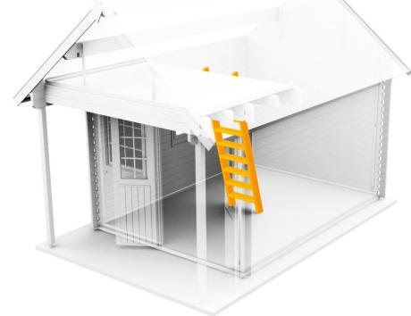
SET THE STAIRCASE AT THE RIGHT SPOT, ATTACH THE FIRST HALF OF THE LADDER FITTINGS TO THE WALL WITH SCREWS.93%
