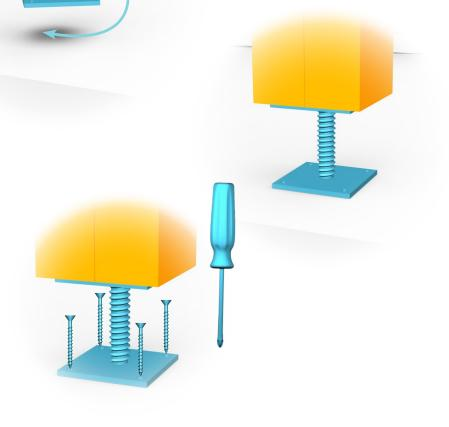
DEPENDING ON THE SURFACE USE SCREWS OR ANCHOR BOLTS TO ATTACH THE POST FOOT TO THE GROUND. 38%
