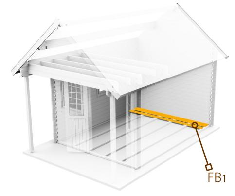
10 SCREWS INTO THE FIRST FLOORBOARD,
